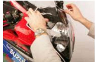
Once the piece is correctly aligned, gently lift the centre section slightly and rinse the Slip Solution out using the Fixing Solution. Lower the film back into place and tack the centre section into place using your squeegee, starting at the centre and working both upwards towards to top of the nose cone, and then downwards towards the lower end.
