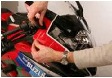
Gently stretch the film to align with the edges of the nose cone, ensuring that your hands are wet with Slip Solution at all times.
