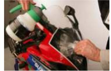
When working on large areas, only apply the Fixing Solution to the section of film that is to be affixed immediately. Leaving the Slip Solution under the film until final fixing will allow it to be repositioned and stretched as required without damaging the adhesive.
